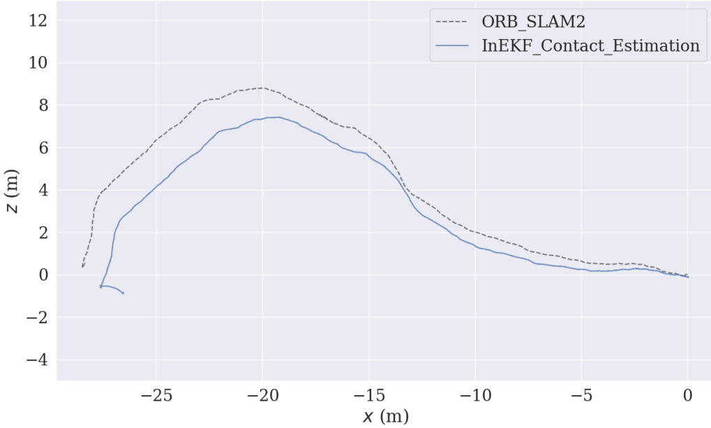
Figure 6: Trajectory of the forest test set. ORB SLAM2 fails close to the end of the sequence. This figure confirms the complementary role of the proposed proprioceptive state estimator.
