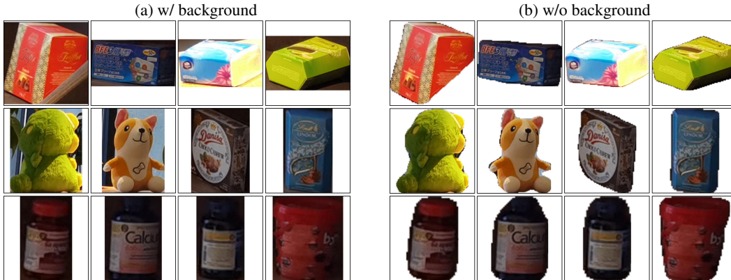
Figure 3: Examples of input proposals to DINOv2_f . Based on a proposal given by SAM, we crop the instance using the minimum bounding square ((a) w/ background) or using the segmentation mask ((b) w/o background) before computing the features.
