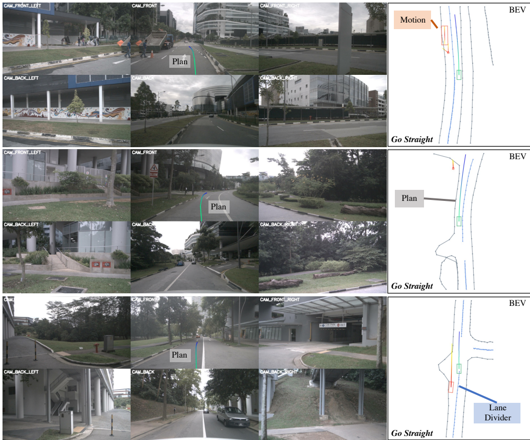
Figure 3: Qualitative results of DiFSD under “Go Straight” driving command in interactive scenes. In the first row, the pedestrian and the construction vehicle are selected as the closest in-path agents for motion prediction and interactive planning, thus DiFSD adjusts the planned trajectory from afar to avoid a collision. In the second row, DiFSD notices the pedestrian in the distance and plans the future trajectory taking the pedestrian intention into consideration. In the third row, DiFSD completes interactive decision-making in the “Cut-in” scenario, and outputs the planned trajectory constrained by the lane divider.
