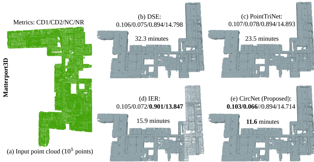
Figure B: Reconstructed scene meshes of different learning-based triangulation methods. We compare their surface quality using the metrics CD1, CD2, NC, and NR. It can be seen that the mesh of CircNet has the lowest Chamfer distances.
