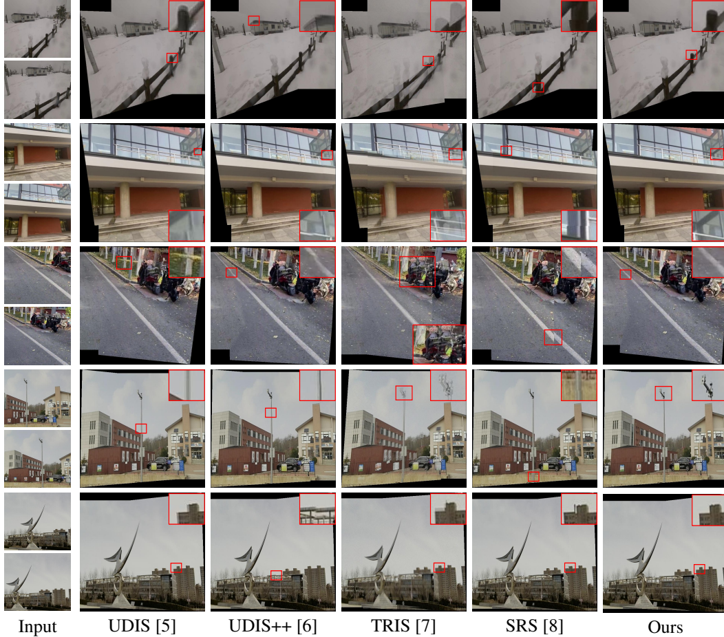
Figure 2: Visual comparison between deep learning based stitching methods and the proposed method on UDIS-D and IVSD datasets.
