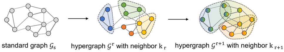
Figure 2: The construction of hierarchical hypergraph. Starting from a standard graph \mathcal{G}_s constructed using rsFC as the adjacency matrix, hypergraphs with different aggregation levels \mathcal{G}^r are built using a k -hop method. As the number of neighbors k_r increases, each node (fMRI signal of a certain ROI) integrates more intra-regional and, gradually, inter-regional information (with different brain regions’ information represented by different colors).
