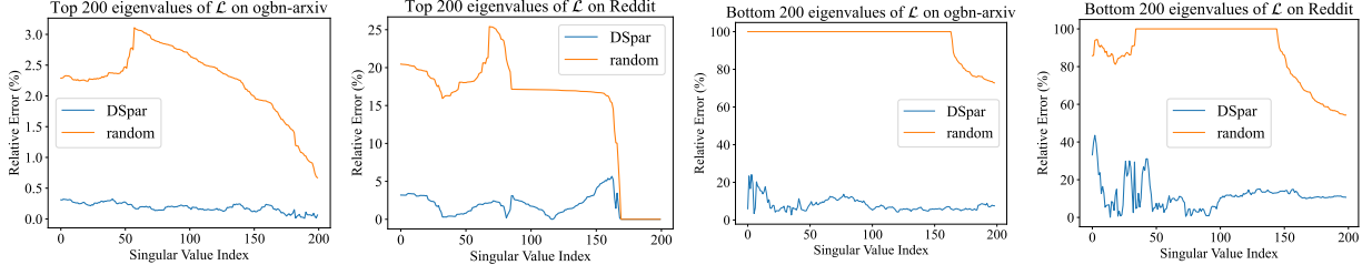
Figure 5: The relative error of the top and bottom eigenvalue of \mathcal{L} , i.e., \frac{\lambda_i - \lambda'_i}{\lambda_i} , sparsified by different methods.
