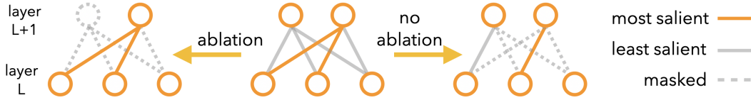
Figure 2: Neuron ablation. At sparsity levels over 90%, RigL learns to completely mask (ablate) a large number of neurons within each layer, effectively reducing layer width. Imposing a constant fan-in constraint requires all neurons to have the same number of (non-pruned) incoming weights and therefore inhibits ablation, which results in worse generalization performance than RigL. Allowing SRigL to ablate neurons restores RigL-level performance.
