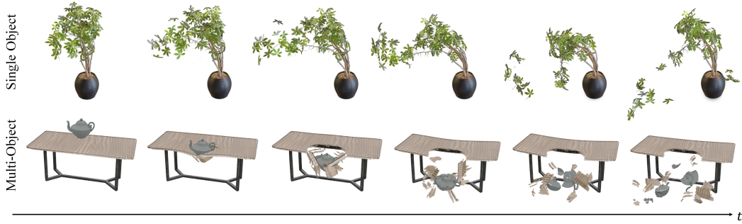
Figure 1: Two extreme mechanical collision scenarios are simulated using our proposed framework: (1) single-object impacts against wind, and (2) multi-object collision interactions with complex fracture dynamics. Notably, the flowerpot object comprises heterogeneous materials (with distinct properties for leaves, stems, and the pot itself), and the table object consists of legs and tabletop, while other teapot is modeled as homogeneous materials.
