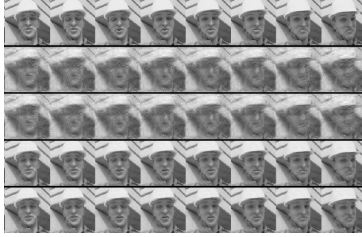
Figure 13: Comparison of reconstructed Foreman video frames. Row 1: ground truth. Row 2: traditional CS with \zeta = 0.1 . Row 3: MSR with \zeta = 0.1 . Row 4: traditional CS with \zeta = 0.5 . Row 5: MSR with \zeta = 0.5 .
