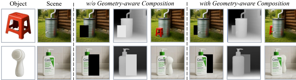
Figure 7: Effect of geometry-aware composition. We sequentially present the masked scene, depth map, and synthesized images, with and without applying geometry-aware composition.
