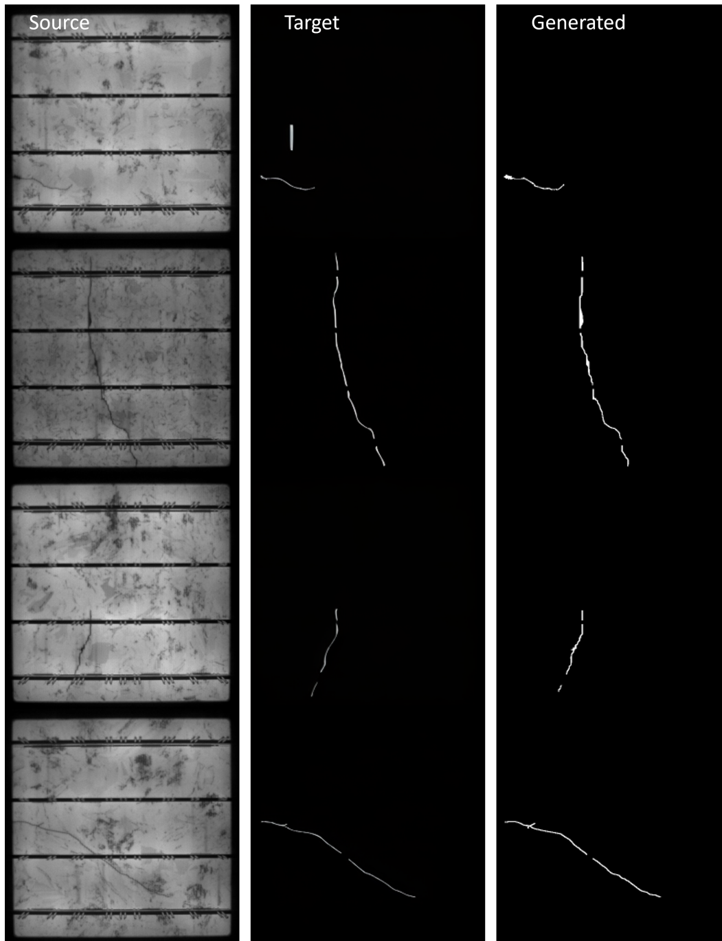
Figure 8: Visualization of the Electroluminescence to Semantic mask translation task; samples are randomly picked from the testing dataset.
