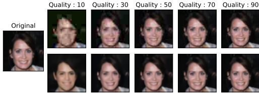
Figure 4: JPEG + noise: results for different compression level (Top: Corrupted; Bottom: Restored).
