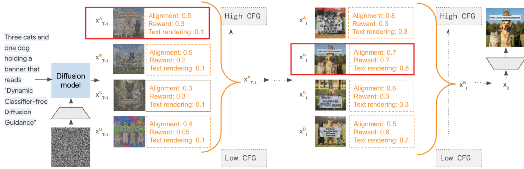
Figure 1: Dynamic CFG. We propose to perform a greedy search over multiple CFG scales and select the one that maximizes the latent evaluators’ scores at each sampling step. The evaluators are small-scale and operate directly in the diffusion latent space increasing the computational overhead during inference by only 1%. Finally, for combining scores by multiple evaluators, we propose an adaptive weighting dependent on the denoising timestep.
