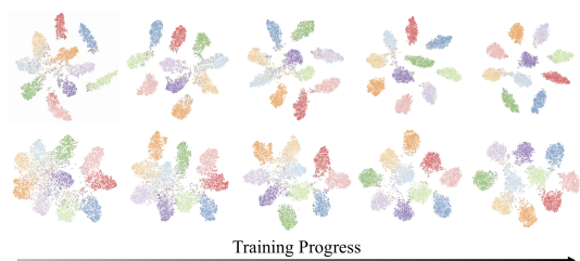
Figure 5: T-SNE progression for speech (top row) and categorical (bottom row) models with ResNet-110 image encoder. From left to right, the plot shows 10%, 30%, 50%, 70%, and 100% progress in training. The speech model develops distinctive clusters at an earlier stage and has better separated clusters overall.
