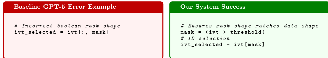
Figure 3: Comparison of array indexing: the baseline code fails due to a shape mismatch in boolean indexing, while our system validates shapes and applies correct masking.
