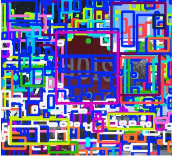
Figure 1: (First Stage) The network tries to find all boxes that may contain objects. A subset of these boxes is shown here.
