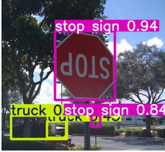
Figure 2: (Second Stage) Final output boxes selected by NMS along with their corresponding labels and confidence scores.
