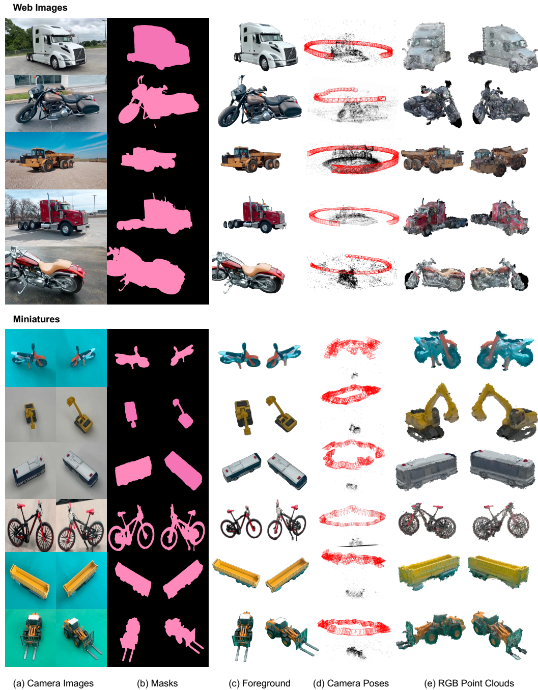
Figure 9: Volumetric 3D rendering Results of RGB Point Clouds.
