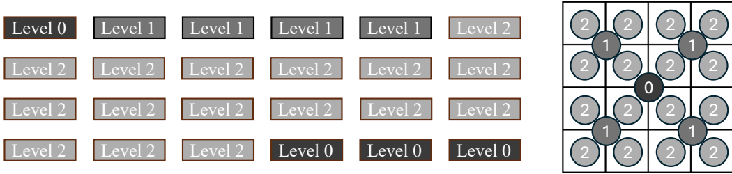
Figure 3: Illustration of hierarchical RoPE allocation in Flux (24 heads). Each rectangle on the left represents the subvector computed by one head, with colors indicating the RoPE level. Black denotes the original patch-level RoPE ( l = 0 ), covers a 256 pixels patch. Level l = 1 corresponds to 64 pixels, and level l = 2 to 16 pixels. The square on the right represents a patch corresponding to one token, illustrating how different levels of positional encodings map to their respective 2D spatial locations, where l = 2 corresponds to a 1/16-sized patch.
