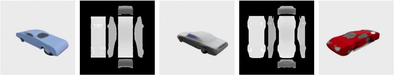
Fig. 2: Traced design lineage across three generations. Left to right: (a) Gen 0 design ( C_d=0.172 ), (b) Gen 0 depth map used for first report card, (c) Gen 1 child addressing rear and wheel weaknesses ( C_d=0.166 ), (d) Gen 1 depth map used for second report card, (e) Gen 2 offspring after further targeted refinement ( C_d=0.118 , 29% improvement over Gen 1).
