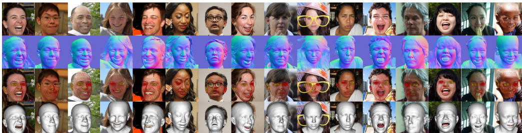
Figure 1: We present Pixel3DMM, a set of two ViTs Dosovitskiy et al. (2020), which are tailored to predict per-pixel surface normals and uv-coordinates. Here, we demonstrate the fidelity and robustness of Pixel3DMM on challenging inputs. From top to bottom we show input RGB, predicted normals, 2D vertices extracted from the uv-coordinate prediction, and our FLAME fitting results.
