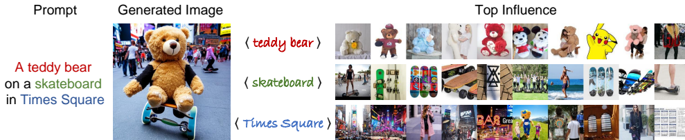
Figure 8: Qualitative results for complex multi-concept attribution using Concept-TRAK. For a generated image from the prompt “ a teddy bear on a skateboard in Times Square ,” Concept-TRAK separately retrieves training samples for each constituent concept <teddy bear> , <skateboard> , and <Times Square> .
