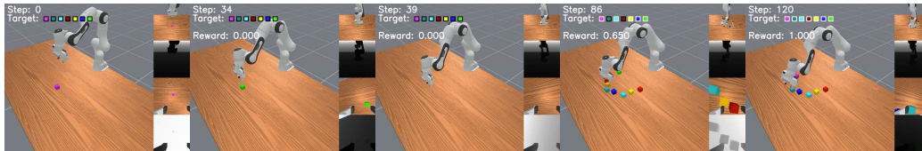
Figure 23: SeqOfColors7-v0 : In front of the agent, 7 cubes of different colors appear sequentially. After the last cube is shown, the agent observes an empty table. Then 9 cubes of different colors appear on the table and the agent has to touch the cubes that were shown at the beginning of the episode in any order.
