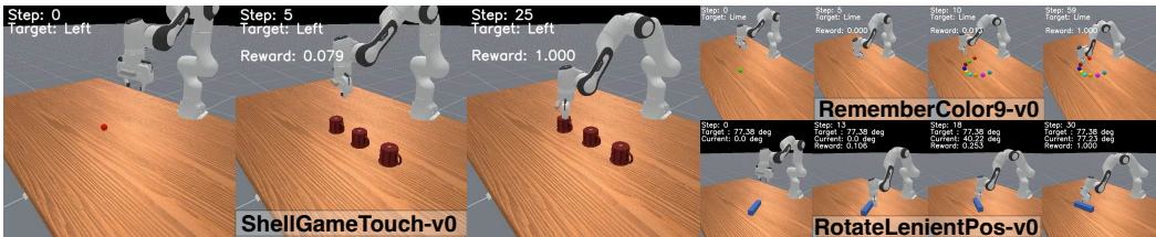
Figure 2: Illustration of demonstrative memory-intensive tasks execution from the proposed MIKASA-Robo benchmark. The ShellGameTouch-v0 task requires the agent to memorize the ball’s location under mugs and touch the correct one. In RememberColor9-v0 , the agent must memorize a cube’s color and later select the matching one. In RotateLenientPos-v0 , the agent must rotate a peg while keeping track of its previous rotations.
