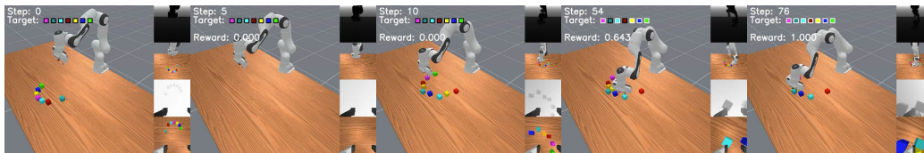
Figure 24: BunchOfColors7-v0 : 7 cubes of different colors appear simultaneously in front of the agent. After the agent observes an empty table. Then, 9 cubes of different colors appear on the table and the agent has to touch the cubes that were shown at the beginning of the episode in any order.
