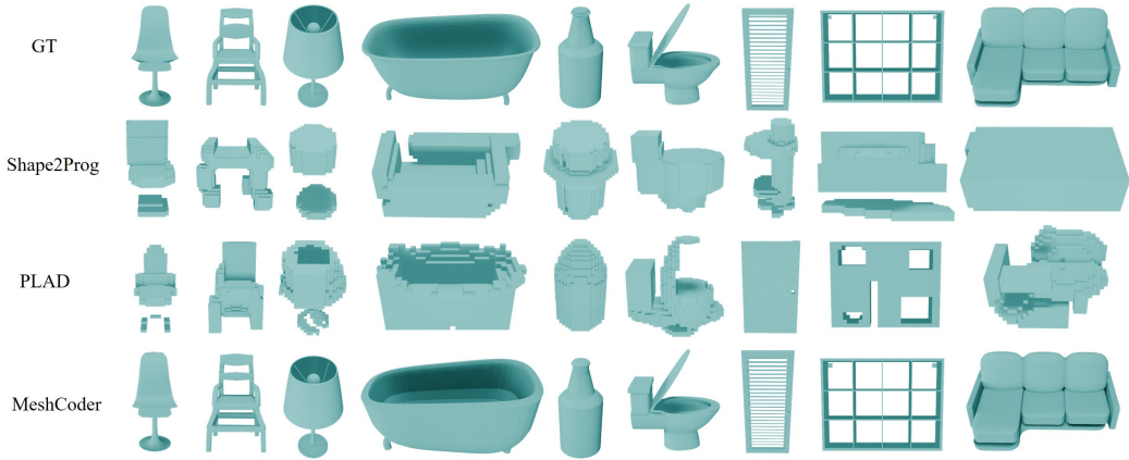
Figure 6: Qualitative comparison of reconstruction performance between MeshCoder and baselines. MeshCoder can accurately reconstruct objects with intricate parts and complex structures.
