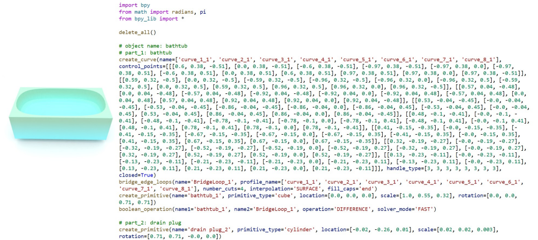
Figure 25: An example of bathtub. The input is a point cloud of a bathtub, and the figure shows the code inferred by the object-to-code inference model, as well as the resulting mesh generated by executing the inferred code.
