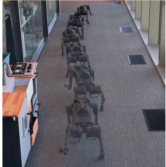
Fig. 7: Real-World Deployment. Frame overlay demonstrating the deployment of the BoT walking policy to a Unitree A1 quadruped robot.
