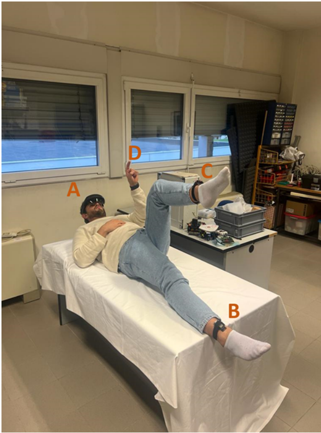
Fig. 7: The experimental setup. (A) the AR headset; (B) the EmotiBit on the right leg; (C) our custom wearable IMU platform on the left leg; (D) the user interacting with the holograms while performing the exercise.
