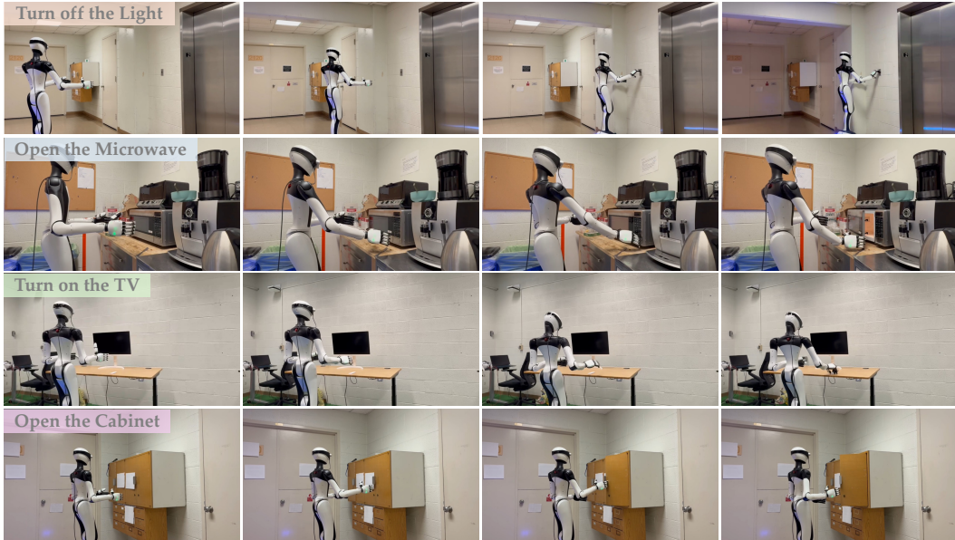
Figure 5: Real Robot experiments on the RobotEra Q5 with a D455, demonstrating four household tasks that require spatial, functional, and part-level interactive elements reasoning for task execution.
