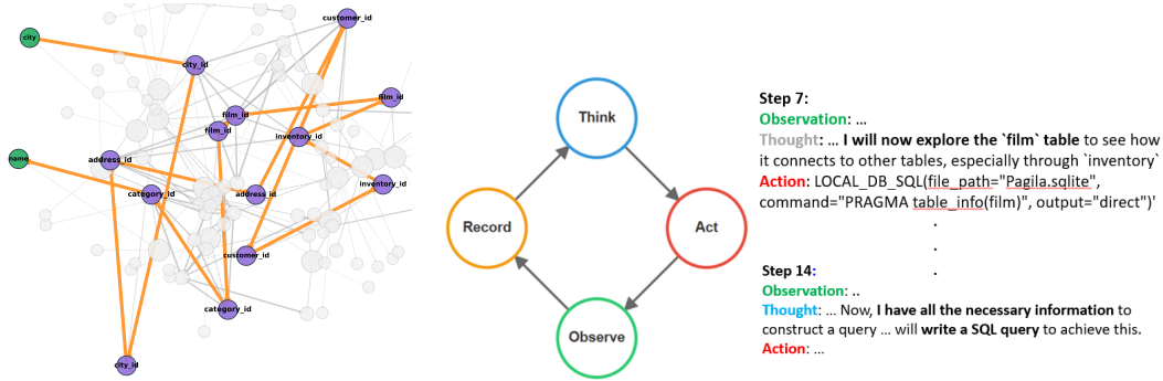
Figure 4: Left: Schema path identified by QAFD-RAG for SQL generation on query local1039 (Lei et al., 2025). Right: Stepwise schema exploration for the same query using Spider-Agent (ReAct) (Lei et al., 2025). QAFD-RAG discovers the full reasoning path in one pass, sharply reducing LLM calls. In contrast, Spider-Agent incrementally explores the schema, requiring 14 calls and higher latency. This comparison highlights QAFD-RAG’s efficiency and accuracy on complex multi-hop queries.
