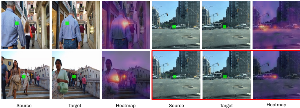
Figure 6: Heatmaps from forwarded feature perturbation. Features are perturbed at green squares in Source, which are also depicted in Target at the same location to highlight the motion between frames. Midway Network without gating units exhibits identity bias (bottom right, red border).
