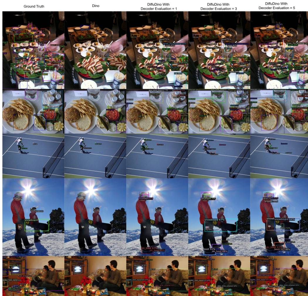
Figure 7: Qualitative comparison of object detection results on LVIS validation set across different numbers of decoder evaluation steps ( t = 1, 3, 5 ), showing DiffuDINO, baseline DINO with ResNet-50 backbone, and ground truth annotations. Only predictions with confidence scores above 50% are shown.
