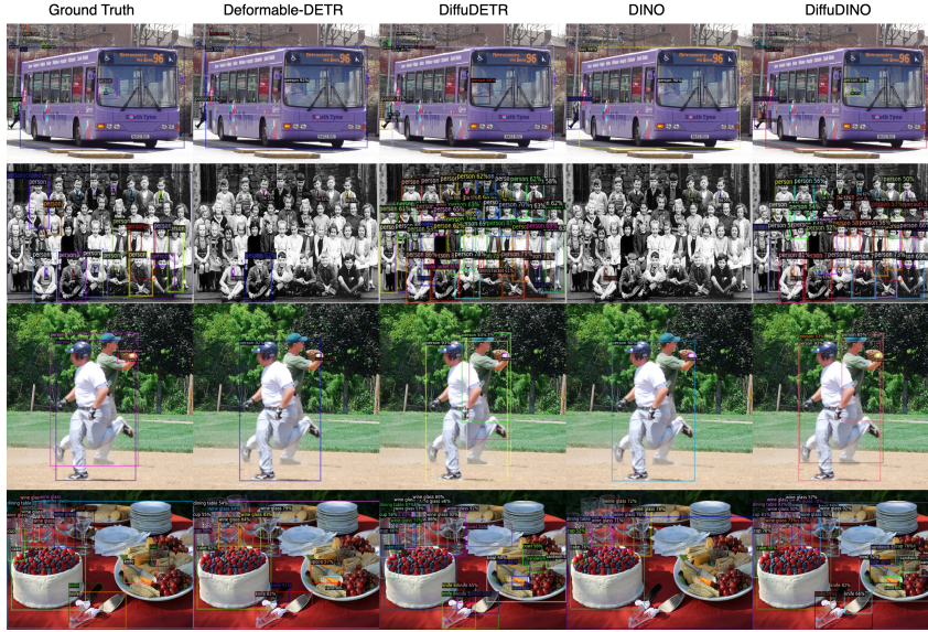
Figure 4: Qualitative comparison between Deformable DETR, DiffuDETR, DINO, and DiffuDINO on COCO 2017 Validation set. Only predictions with confidence scores above 50% are shown.
