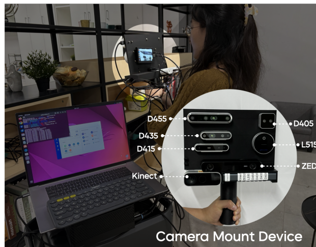
Figure 5: Multi-camera mount device for capturing the color-depth image pairs from multiple depth cameras all at once. In practice, we use two computers to capture all the data due to the USB bus bandwidth limits.
