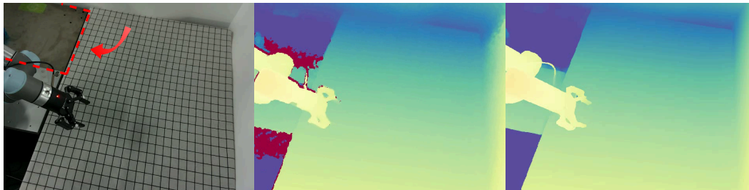
Figure 22: A typical failure case of CDM-L515 , caused by the wrong prompt and the less informative semantic information contained in the RGB image.
