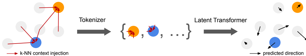
Figure 3: Architectural adaptation. MoGen injects local geometric context by finding the k -Nearest Neighbors ( k -NN) for each point and appending their relative coordinates as features. This information, along with the point’s own coordinates, is processed into tokens that attend to a set of latent tokens in a transformer architecture, enabling the generation of high-fidelity morphology. The model predicts for each point the direction it will move into during integration.
