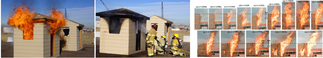
Figure 2: Left: Real-world combustion in a live-fire drill (5280 Fire Science); Right: Full-scale combustion test measuring flame spread time (Zhang et al., 2021)
