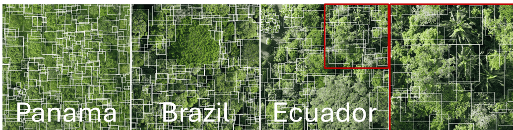
Figure 1: The SELVABOX dataset. The illustrated samples are extracted from rasters recorded in Panama, Brazil and Ecuador with a spatial extent of 80\text{m} \times 80\text{m} and a resolution of 1.2 to 5.1 cm per pixel. The red square on the right highlights a zoom of the Ecuador sample with a spatial extent of 40\text{m} \times 40\text{m} at the same resolution.
