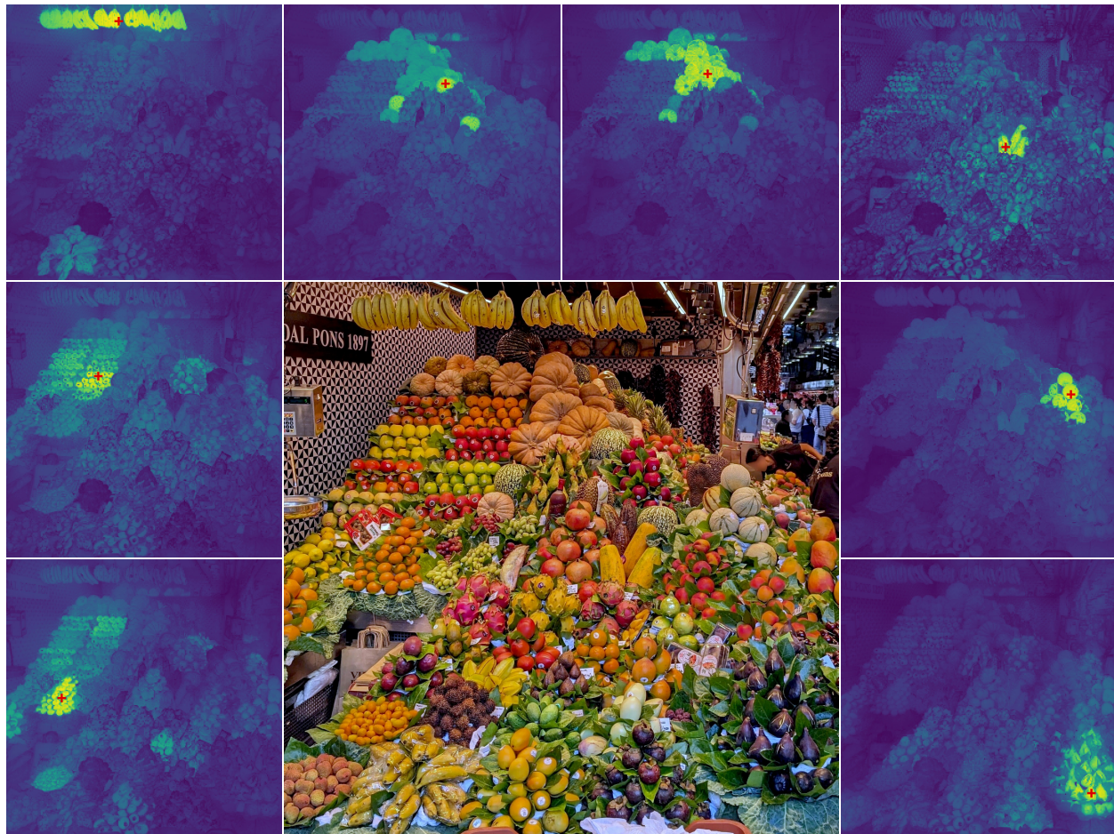
Figure 3: High-resolution dense features. We visualize the cosine similarity maps obtained with DINOv3 output features between the patches marked with a red cross and all other patches. Input image at 4096 \times 4096 . Please zoom in, do you agree with DINOv3?
