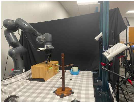
Figure 6: Hardware Setup. We deploy our method on a Franka Emika Panda robot.
