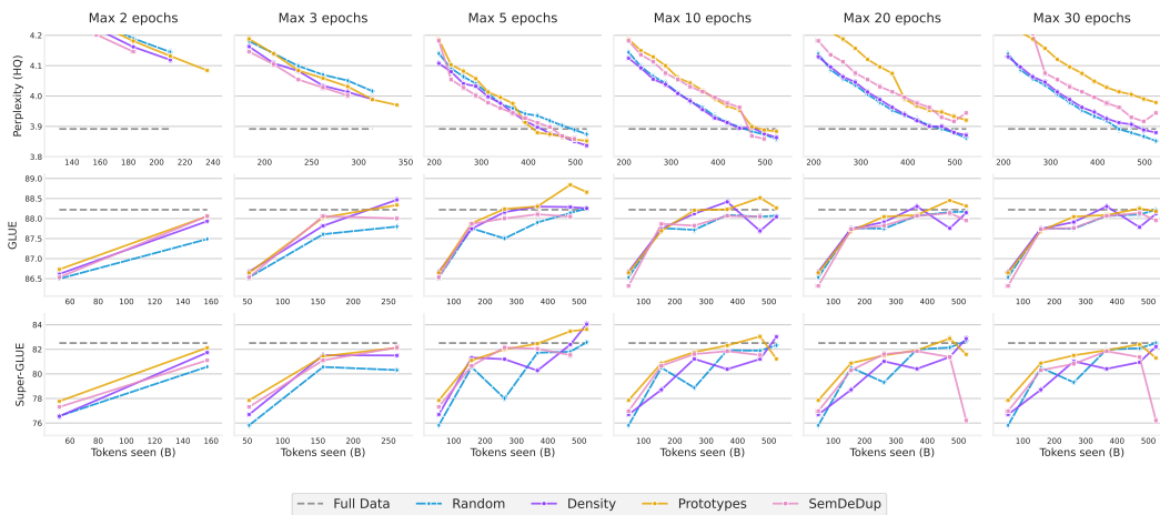
Figure 22: Average data-efficiency of pre-training T5-Large on sampled data, stratified by maximum number of allowed repetitions on the sampled dataset. Each point in this plot represents the performance of an intermediate checkpoint averaged over all sampling ratios, as long as the maximum allowed repetitions have not been reached. See Section F for a description about the metrics used in this plot.
