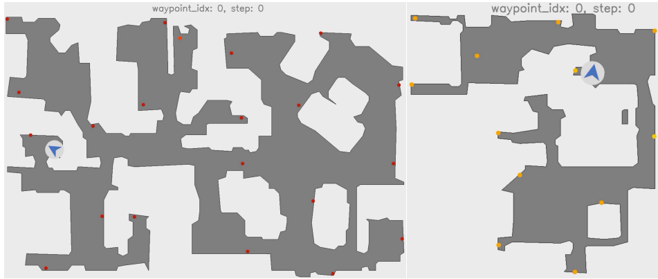
Figure 12: Top-down visualization of sampled waypoints in a scene. Red (left) and yellow (right) dots are the final waypoints after radius-based pruning. The proposed strategy places waypoints throughout peripheral regions while avoiding redundant interior points, yielding diverse and spatially balanced trajectories.
