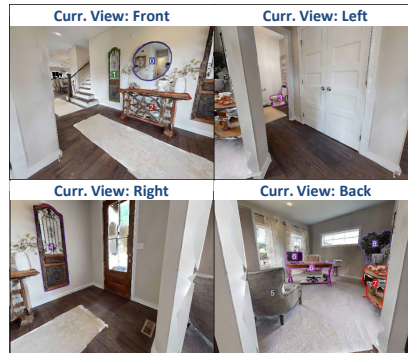
Figure 10: Illustration of the Set-of-Marks (SoM) representation that encodes candidate navigable directions. The high-level planner chooses among these discrete landmarks when constructing candidate action plans.
