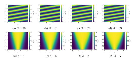
Figure 5: The solution profiles at PINN failure modes: (a), (b), (c) and (d) for  $\beta \in [30,40]$  with initial condition  $1+\sin(x)$  and (e), (f), (g) and (h) for  $\rho \in [1,10]$  with initial condition  $\mathcal{N}\left(\pi,\left(\frac{\pi}{2}\right)^2\right)$ . The solution profile is constructed using the union of 1,000 test prediction points and the remaining ground truth points.
