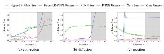
Figure 3:  $L_2$  relative error measured at unseen parameters for (a) convection, (b) diffusion, and (c) reaction. The result of seen parameters are plotted together. The grey area indicates the region where the model extrapolates the coefficient  $\beta$ ,  $\nu$ , or  $\rho$ .
