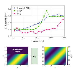
Figure 4: (upper) The  $L_2$  relative error is evaluated for each convection coefficient  $\beta=1.5,2.5,\cdots,19.5$  as an extrapolation task. (lower) The graph illustrates the extrapolation of convection equation with  $\beta=5.5$  at  $0.6 \le t \le 1.0$ .
