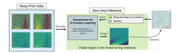
Figure 1: **End-to-end schematic diagram of our model.** Our model performs in-context learning based on the given observations, i.e., context, to infer the solution. Even when trained with noisy prior data, our model can obtain clean solutions due to its Bayesian inference capability.
