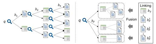
Figure 3: Left: Iterative 3-step retrieval over individual blocks (baseline). **Right:** Fusion 1-step retrieval over fused groups, which greatly lowers the cost of iterative encoding and retrieving.
