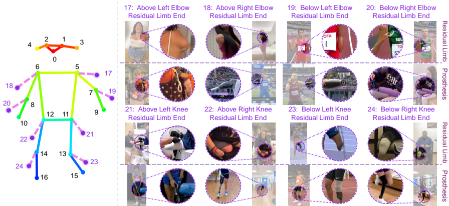
Figure 3: Demonstration of Our Keypoint Schema. Our extended pose definition is built on the MS COCO keypoint schema by adding eight residual limb end keypoints (17 through 24). The left panel shows the full skeleton: original COCO keypoints are connected by solid lines, and the eight new residual limb end keypoints are marked as purple circles. The right panel presents, for each residual limb end keypoint, a cropped view of a subject with the corresponding amputation and a matching view of the same subject wearing a prosthetic device.
