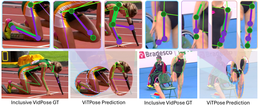
Figure 7: Case study of ViTPose (ViT-B) predictions trained on InclusiveVidPose. We highlight incorrect keypoints and skeleton segments in bold, demonstrating the challenges introduced InclusiveVidPose. Residual-limb endpoints appear in purple, and all other keypoints appear in green.
