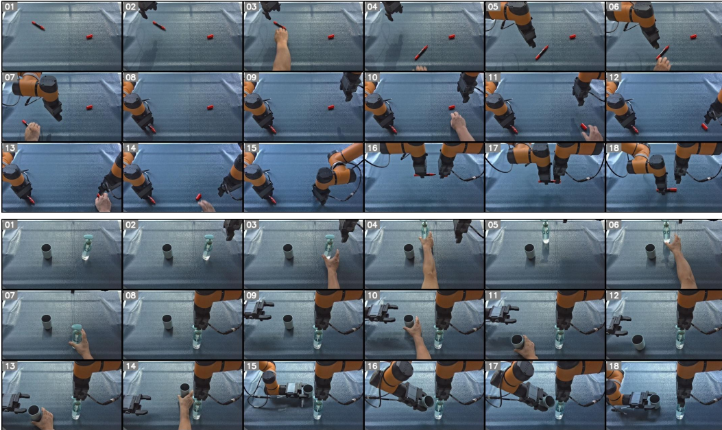
Figure 9: Examples of plugpen (top) and pressing (bottom) show that under the uneven lighting, the system is subjected to consecutive external interferences, and tasks can still be completed.
