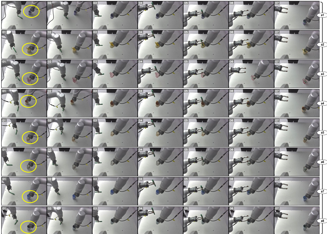
Figure 15: Taking the inserting task as an example again, we changed the cup being grasped by the right arm to cups of completely different shapes (including mugs with handles in examples a1/a2/a3/a4 , and ordinary cups without handles in examples a5/a6/a7/a8 ). These newly added objects are circled in yellow color. We found that VLBiMan can still successfully locate the objects using our designed method of using the foremost point of contact between the object and the table as a representative point (note that at this time, it is not necessary to use the orientation estimation method to estimate the object’s pose again), thus helping to stably grasp these cups and ultimately complete the inserting task objective.
