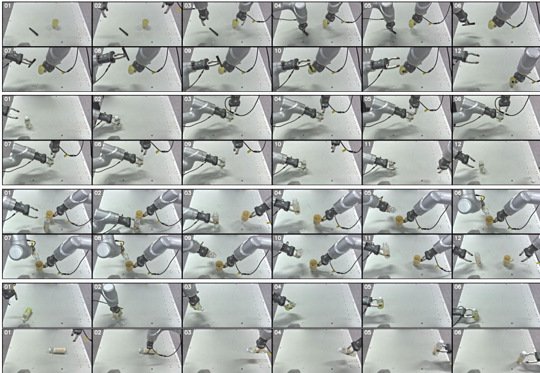
Figure 12: Examples of four transferred bimanual tasks with synchronized dual-arm movement. Segments from top to bottom are tasks inserting, unscrew, and pouring, which have relatively high dual-arm synchronizability. The last row are examples of single-arm task reorient, explicitly examining left- or right-handed execution strategies.
