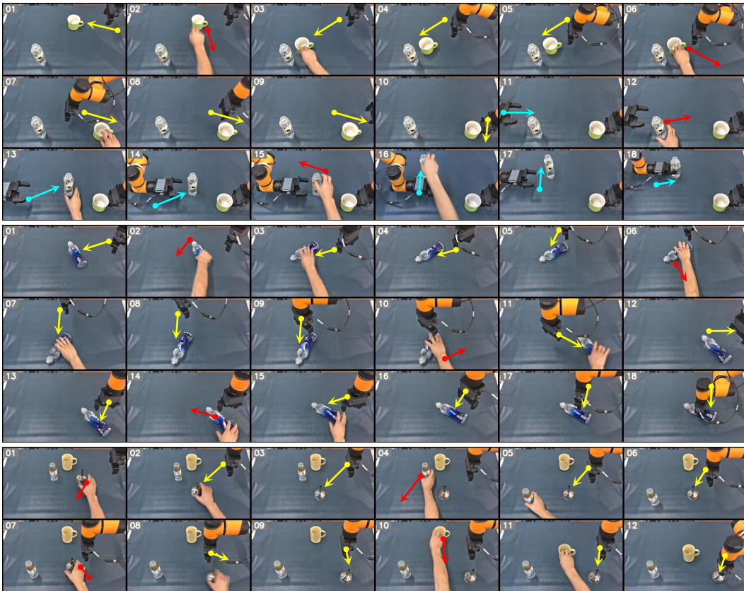
Figure 11: Example of dynamic interferences during task execution. From top to bottom, they are segments of the dynamic closed-loop grasping phase of tasks pouring , reorient+unscrew , and tool-use funnel , where each object is manually disturbed from one to three times. The red arrow indicates the direction of the manually moved object (interfering). The cyan arrow and yellow arrow indicate the movement direction of the left and right robotic arms (chasing) respectively.
