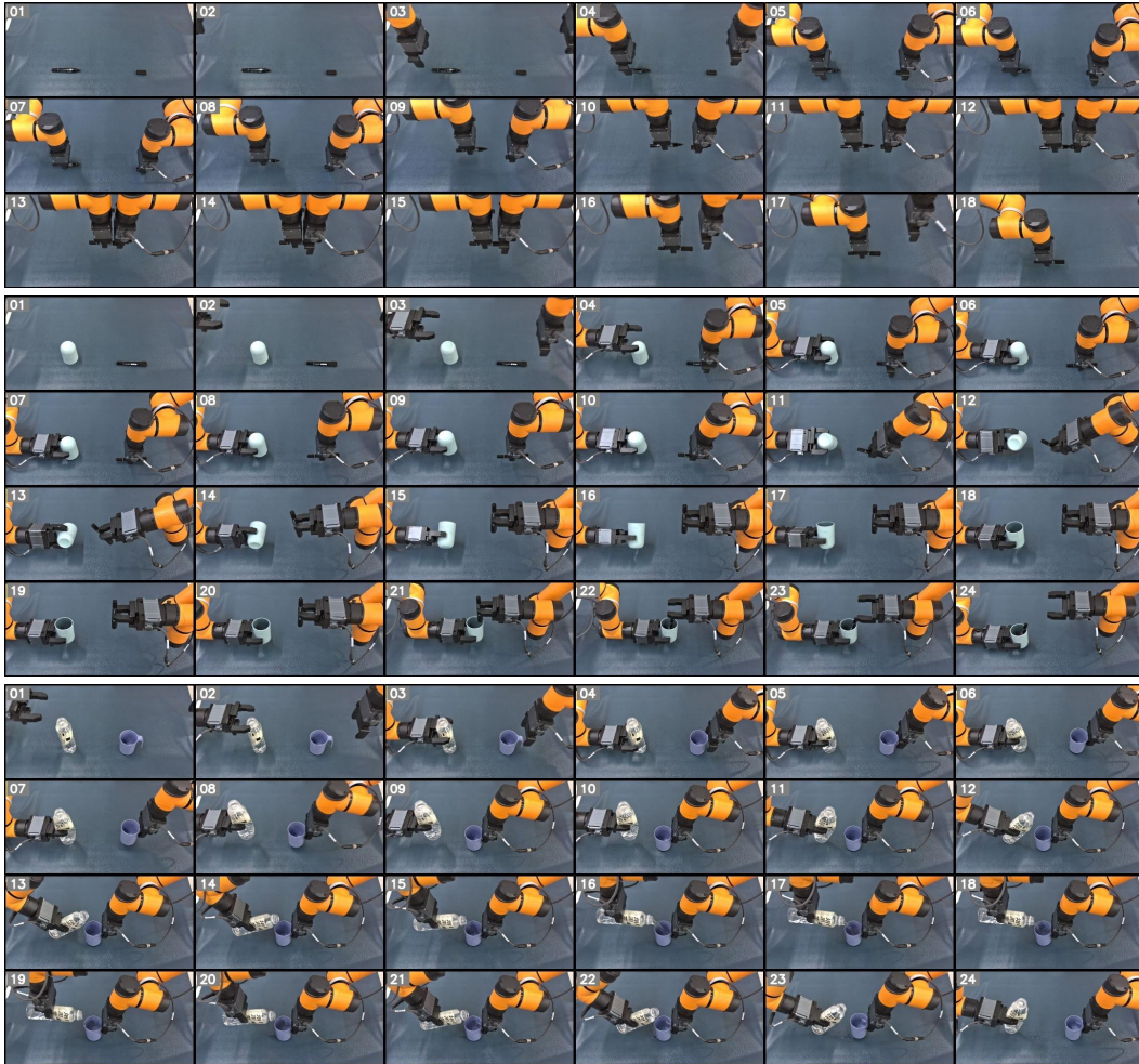
Figure 10: Examples of synchronized dual-arm movement. Segments from top to bottom are tasks plugpen , inserting , and pouring , which have relatively high dual-arm synchronizability.
