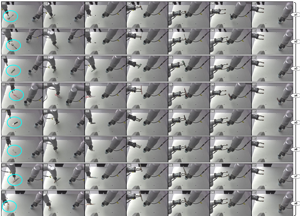
Figure 14: Taking the inserting task as an example, we replaced the marker pen held by the left arm with other rectangular objects that were completely different (including spoon in cases a1/a2 , brush in cases a3/a4 , spatula in case a5 , syringe in case a6 , and toothbrush in cases a7/a8 ). These newly added objects are circled in cyan color. We found that VLBiMan could still successfully locate the objects based on our designed method of using the centroid of the object’s 2D mask as a representative point. Furthermore, it accurately estimated the object’s pose using the orientation estimation method in Algorithm 1, thereby helping to stably grasp these objects and ultimately achieve the inserting task objective.
