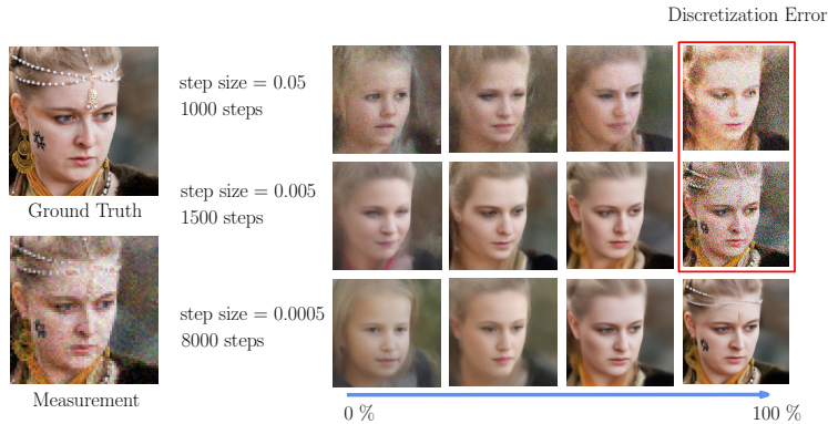
Figure 9: Unadjusted Langevin Algorithm (ULA) with different step sizes. Larger step sizes accelerate convergence but introduce greater discretization error, substantially degrading sample quality.
