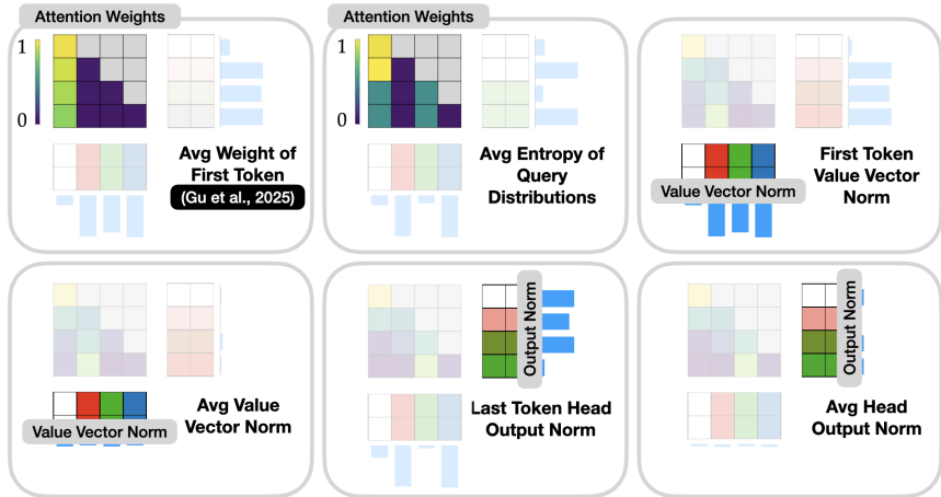
Figure 1: Score Functions for Inactive Heads. Our simple score functions measure all three components of attention: attention weights, value vectors, and head output vectors. In each cell, we give an example of the type of attention head that would be identified by each score function once scores are thresholded. For attention weights, the colorbar displays weights. For vectors, color represents direction, and length of the blue bar represents magnitude. For example, the Avg Weight of First Token score (Gu et al., 2025; Guo et al., 2024a) is calculated by computing average weight to the first token, and heads that exhibit high attention to the first token are identified if their their score exceeds a threshold. Value vectors and head outputs do not play a role, which we illustrate with a fade. Including normalized versions of these 6 score functions, there are 12 in total.
