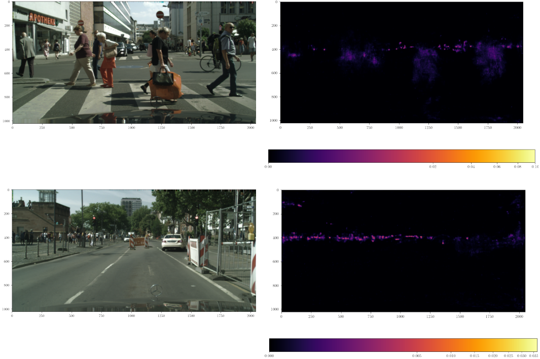
Figure 4: Visualization of ensemble intensity variance on two Cityscapes street scenes. We observe similar behavior as for individual models, where intensity for objects in the distance are sharply peaked, just as the standard deviations computed here. The top image shows how objects close to the ego car have medium variances spread out over a larger area.
