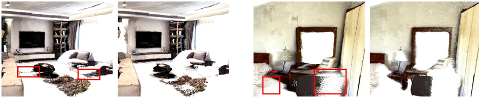
Figure 11: Before-and-After Visualization of the Adaptive Erosion Strategy. The method effectively removes noisy points and preserves high-confidence regions, producing cleaner and more consistent geometries.
