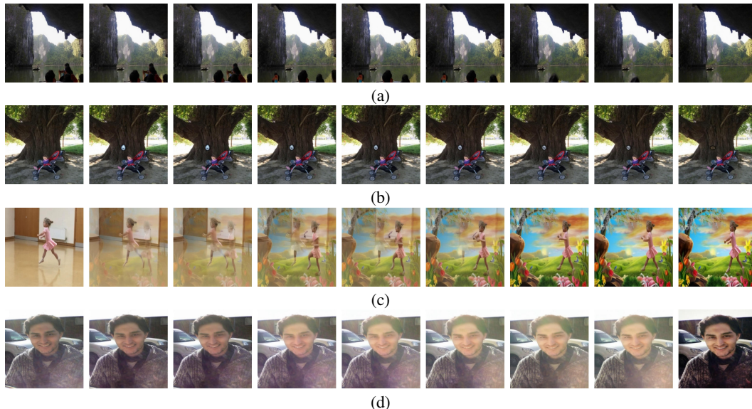
Figure 5: Uncontrollable predicted intermediate frames examples of diffusion-based FI models. Samples (a) and (b) show an unexpected object prediction, while samples (c) and (d) show an unexpected motion generation.
