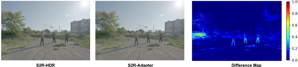
Figure 9: Difference maps of models trained on the rendered dataset (S2R-HDR) before and after domain adaptation (S2R-Adapter) to the SCT dataset. The differences are primarily concentrated in texture-rich regions such as trees, grass, and people, while ground, sky, and buildings remain largely unchanged. This highlights that the key domain discrepancies lie in fine textures and demonstrates the effectiveness of domain adaptation in bridging the domain gap.
