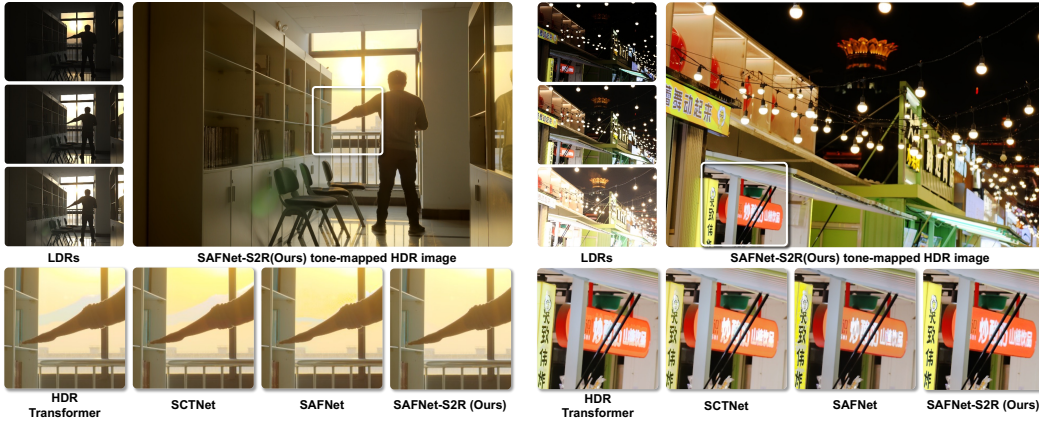
Figure 7: Visual results on real-captured scenes show our solution reduces ghosting in backlit scenes (left) and recovers highlights (right).
