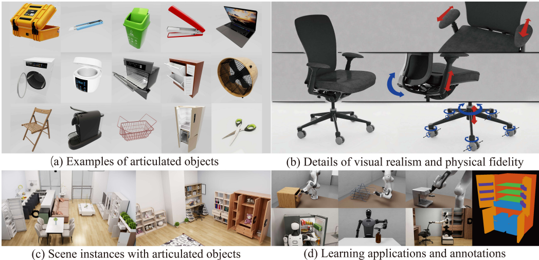
Figure 1: ArtVIP spans 9 categories, 37 subcategories, and 992 digital-twin articulated objects. (a) Representative assets across categories and articulation types. (b) High-fidelity physics enables realistic interactions; for example, when pushing an ergonomic chair, its casters rotate accordingly. (c) Six sim-ready scenes in which all objects support real-world-consistent interactions. (d) Pixel-level annotations and sim2real evaluations.
