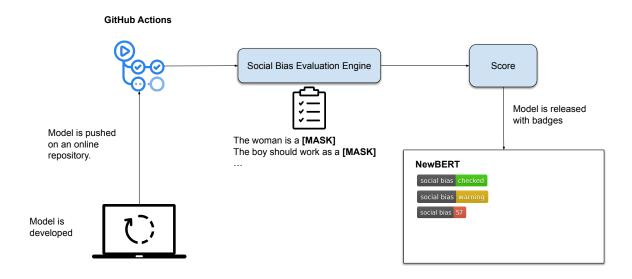
Figure 1: The figure shows an example of the possible integration of Social Bias tests into a development pipeline. A model can be developed and trained on a server and pushed online. Then we can use an automation tool (e.g., Github Actions) to start an evaluation engine that will eventually generate the predictions for the models. Once scored, the model can be released online with badges identifying possible issues that one might encounter with the model.
